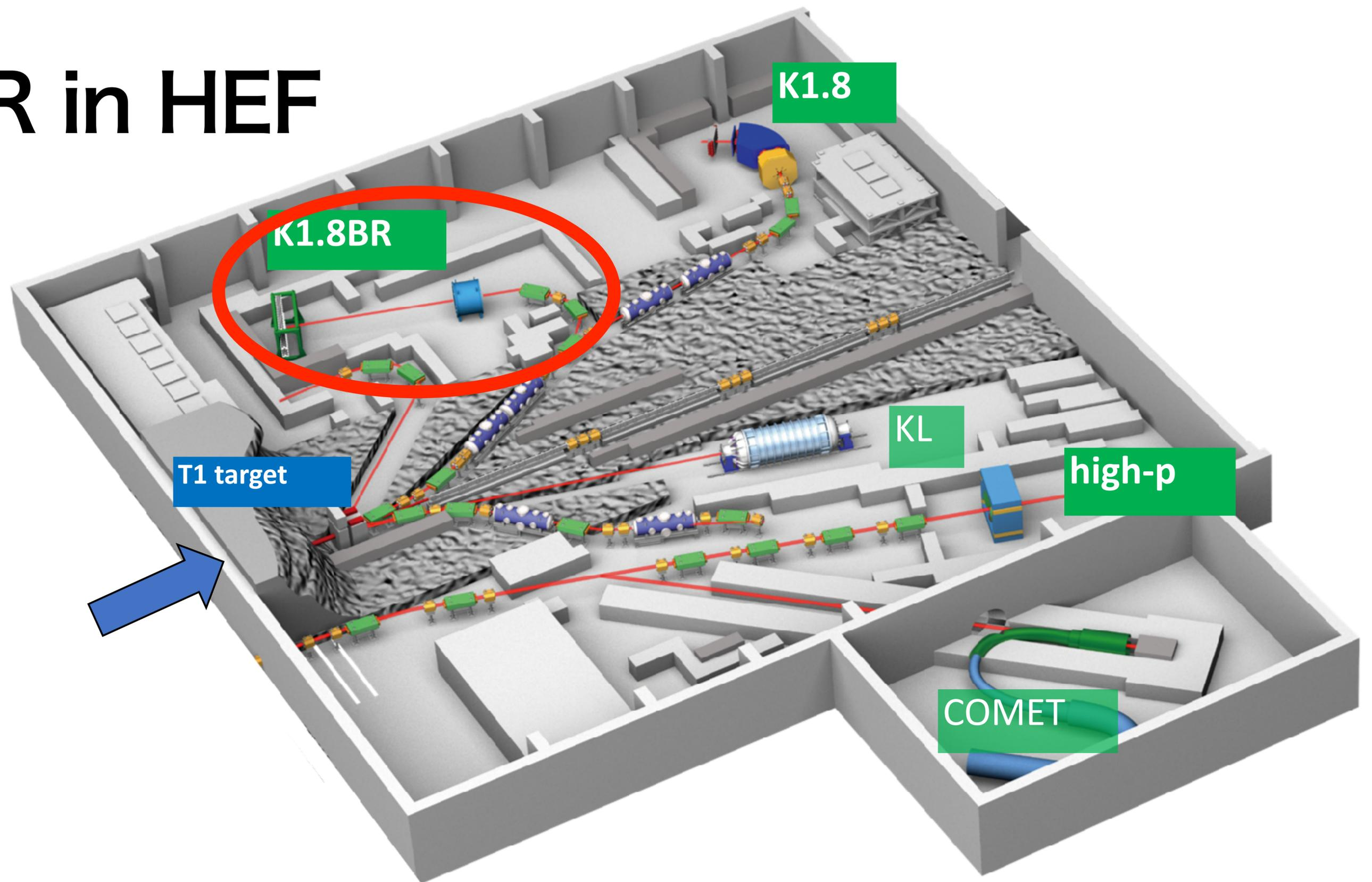
K1.8BR suitable for low-energy K- beam below 1 GeV/c
