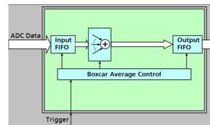
The Boxcar average or high-resolution mode is a form of averaging. The ADC oversamples the signal and averages neighboring points together. This mode uses a real-time boxcar averaging algorithm that helps reducing random noise. It also can
