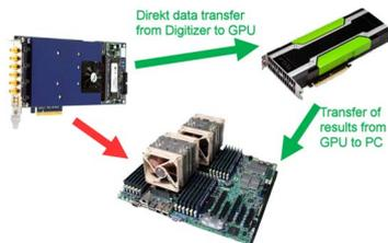
For applications requiring high performance signal and data processing Spectrum offers SCAPP (Spectrum's CUDA Access for Parallel Processing). The SCAPP SDK allows a direct link between Spectrum digitizers, AWGs, DDS or Digital Data Ac-
