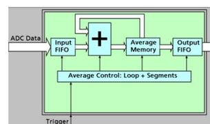
The Block Average Module improves the fidelity of noisy repetitive signals. Multiple repetitive acquisitions with very small dead-time are accumulated and averaged. Random noise is reduced by the averaging process improving
