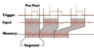
The Multiple Recording mode allows the recording of several trigger events with an extremely short re-arming time. The hardware doesn't need to be restarted in between.
