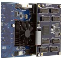
The Star-Hub is an additional module allowing the phase stable synchronization of up to 8 boards of a kind in one system. Independent of the number of boards there is no phase delay between all channels. The Star-Hub distributes trigger and clock information between all boards to ensure all connected boards are running with the same clock and trigger. All trigger
