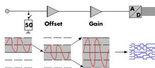
The analog inputs can be adapted to real world signals using a wide variety of settings that are individual for each channel. By using software commands one can select a matching input
