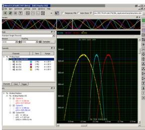
A base license of SBench 6, the easy-to-use graphical operating software for Spectrum cards, is included in the delivery. The base license makes it possible to test the card, display acquired data and make some basic measurements. It's a valuable tool for checking the card's performance and assisting with the unit's initial
