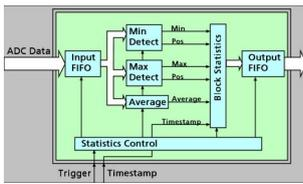
The Block Statistics and Peak Detect Module implements a widely used data analysis and reduction technology in hardware. Each block is scanned for minimum and maximum peak and a summary including minimum, maximum, average,
