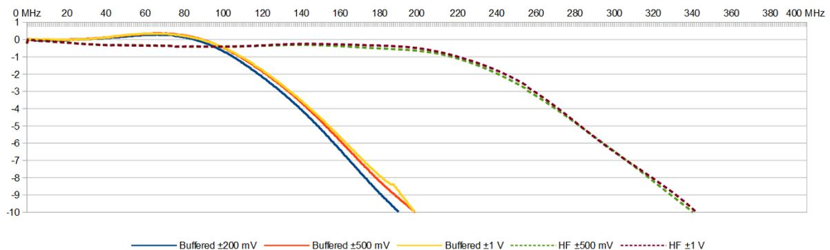
**Frequency Response M4i.442x, M4x.442x, DN2.442-xx, DN6.442-xx and DN2.822-xx**
