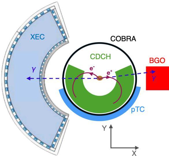
**Fig. 1** Representation of the MEG II apparatus employed for this work. The Cockcroft-Walton proton accelerator is located at a  $z$  position several meters away from the COBRA center.
