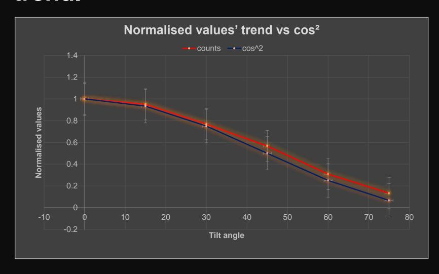
After building the chart, we inserted our data in a graph and verified that the trend is similar to the cosine squared  $(cos^2)$  of the tilt angle of the telescope.
