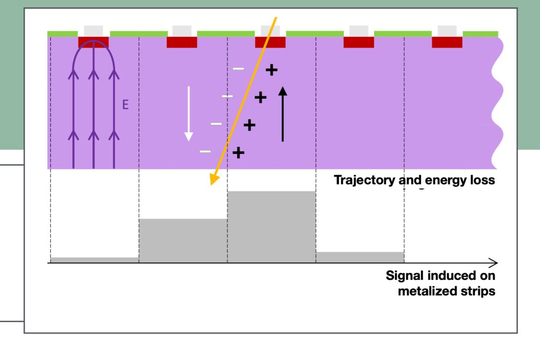
The signal produced on strips by drift-diffusion can be injected to a Silicon sensor equivalent circuit: CAPACITIVE NET
