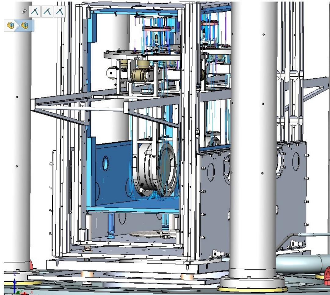
ETpathfinder cryogenic shields: in blue the innermost shield, a 15-K platform, with the mounting rails to transport the cryogenic payloads. All shield panels are omitted here. Design engineering: R. Garcia (IFAE Barcelona), M.Doets, K.Lam, M. Baars (Nikhef), H.J.M. ter Brake, C. Vermeer, M. van Limbeek (EMS Twente), R. Kunst (Demcon)
