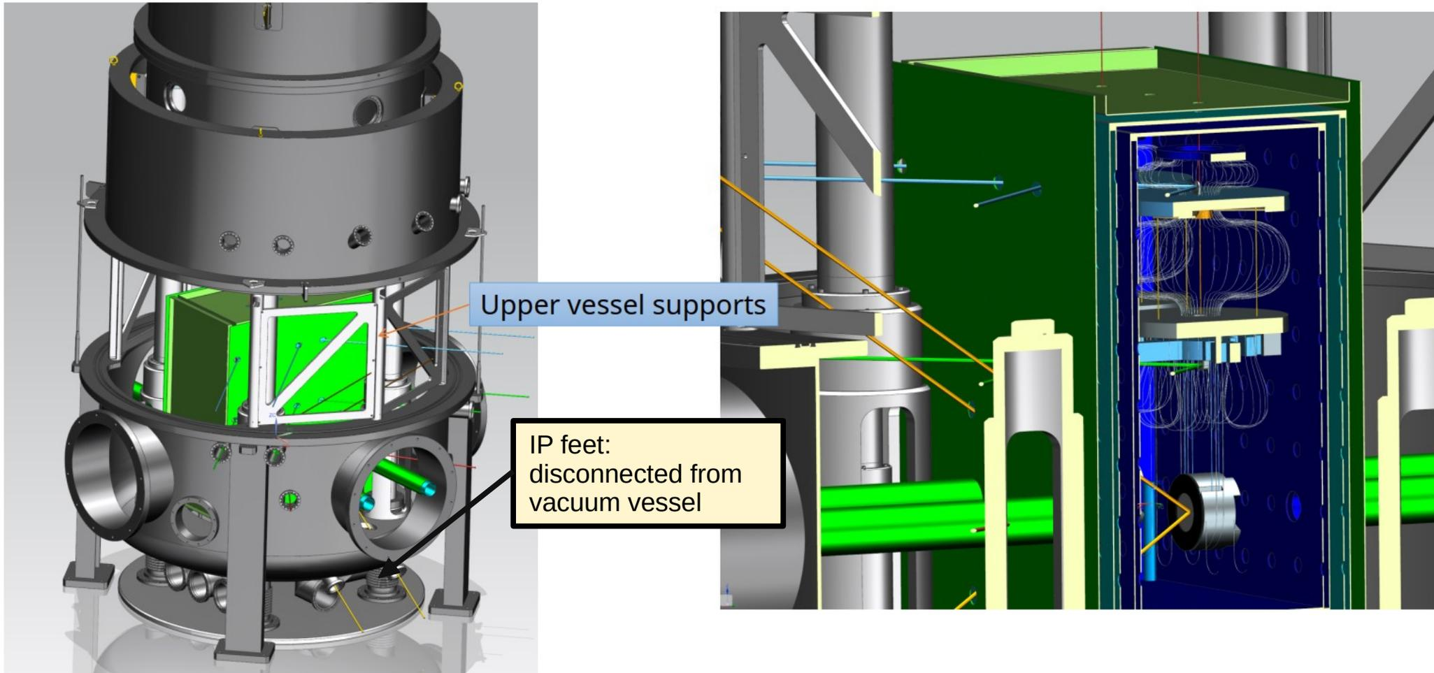
ETpathfinder design, **M. Doets 2019**. Mantle-lifting system for sideways access. Shields in between the inverted pendulum frame and the frame for the upper part of the tower. Inverted pendulum feet connected to stable floor through bellows; tower and suspension are mechanically decoupled so that tower modes do not influence the suspension.
