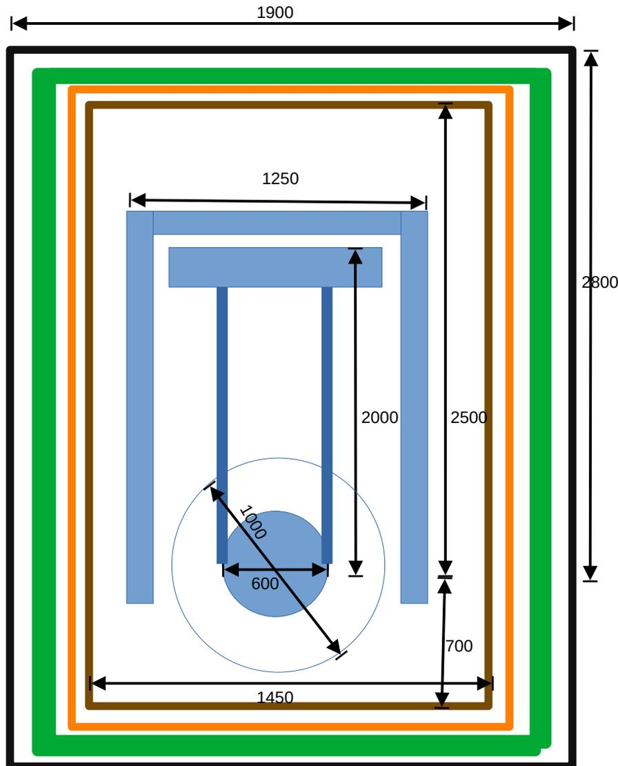
From baseline (see Fulvio contribution 18-02-2025) : assume a mirror diameter of 600 mm (is that really an option in the future?), and 1000mm diameter for the reaction cage/baffle around the mirror; I assume that that is also the diameter for the cold cryolink around the beam.
