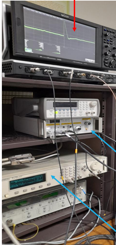
Single pixel CSA output signal with 2 laser pulses
