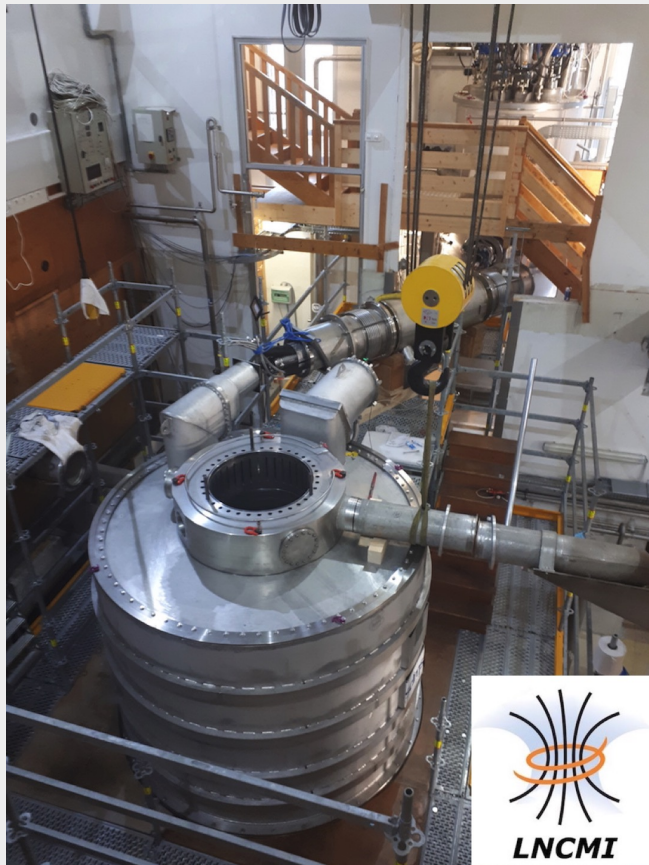
Pilot experiment with a 14 T magnet And 6.4 GHz cavity
