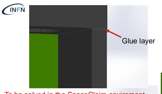
The overall mesh shoud be connected. Use of solid elements also for thin layers.
