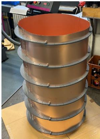
Figure 4: Left: Picture of the DQLF prototype cavity under construction at KIT. Right: CAD model of the design of a second version of the DQLF cavity at CERN.
