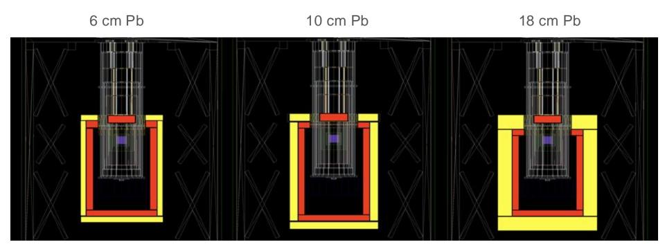
Consider, in all cases, 8 cm of Cu (in red). Thickness obtained from previous simulations, required to reduce OPERA Pb background contribution in BULLKID-DM.
