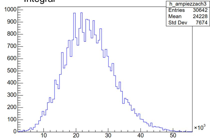
From this we understand that we can **only derive a calibration from amplitudes** and not from integrals, since with integrals we do not have a definition of peaks
