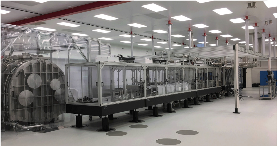
L3-HAPLS with compressor at ELI-Beamlines
