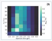
Fig 3 –  $2\omega_L$  conversion efficiency as a function of aperture diameter and initial target density
