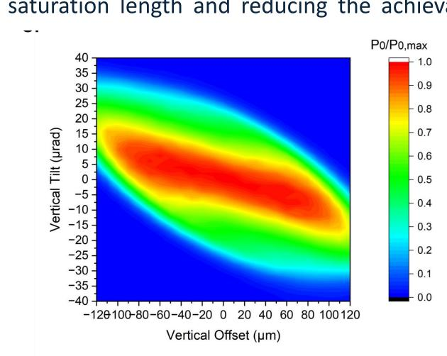
Nominal beam with  $\beta$ =8 m in circular pol.: Maximum achievable radiation power level  $P_0$  normalized to the maximum FEL power  $P_{0,max}$  achieved as a function of the initial horizontal and vertical tilt angles and offsets
