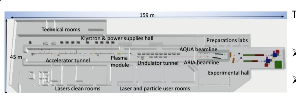
The future EuPRAXIA@SPARC\_LAB FEL facility will host two FEL beamlines driven by the X-band LINAC and a PWFA stage. The two foreseen FELs will deliver short pulses with selectable polarization:
