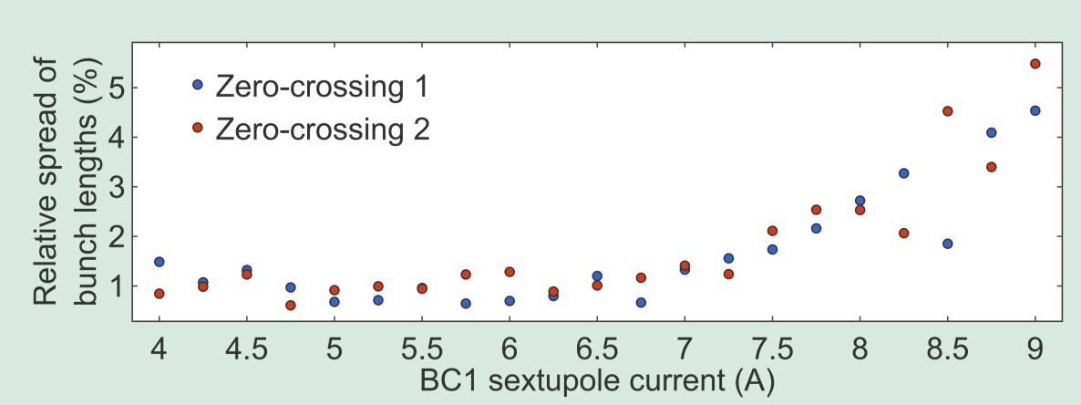
Relative standard error of shot-to-shot bunch lengths as a function of sextupole current ( $T_{566}$ ). For sextupole currents below 7 A, the measured bunch length jitter was constant and finite, determined by the full accelerator system and measurement precision.
