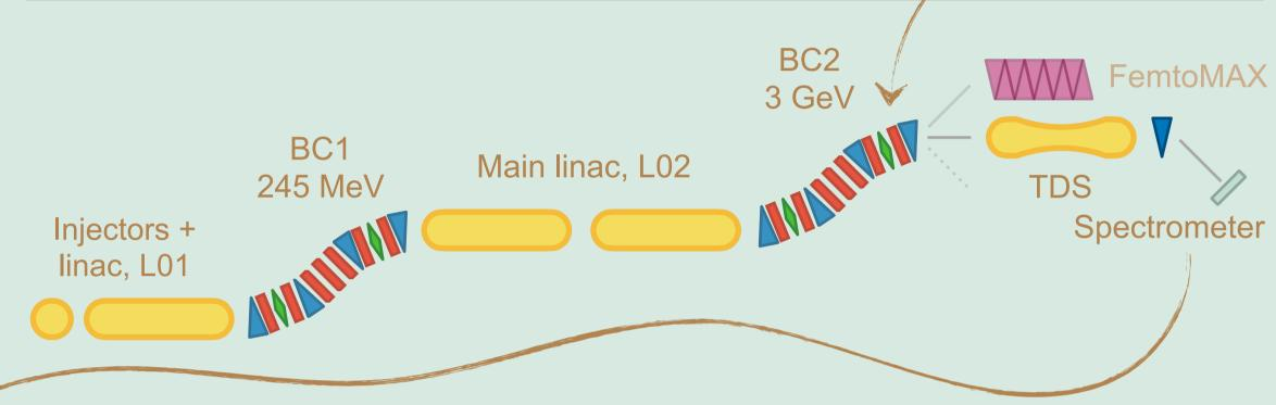
Schematic of the MAX IV linac [4], including the diagnostics beamline with the transverse deflecting structure (TDS) and spectrometer where the bunch current measurements were performed.
