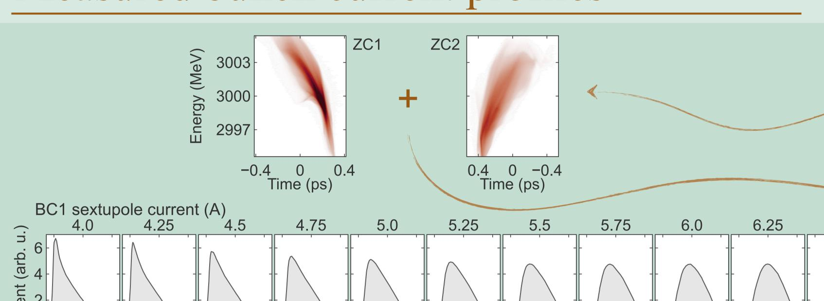
Streaked bunch images from the TDS spectrometer screen along with current profiles reconstructed from measurements of a BC1 sextupole scan using the "two-point tomography" method [5]. The majority of the compression was done in BC1. A narrow range of sextupole strengths yielded a smooth transition from down-ramped to up-ramped bunch currents.
