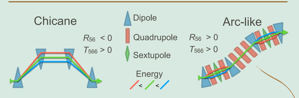
Schematics of different bunch compressor geometries. Chicanes are simple but longitudinal dispersions of different orders ( $R_{56}$ ,  $T_{566}$ , ...) are intrinsically linked. Arc-like compressors [1,2,3] are more complex, but do not require harmonic cavities and dispersions are independent.
