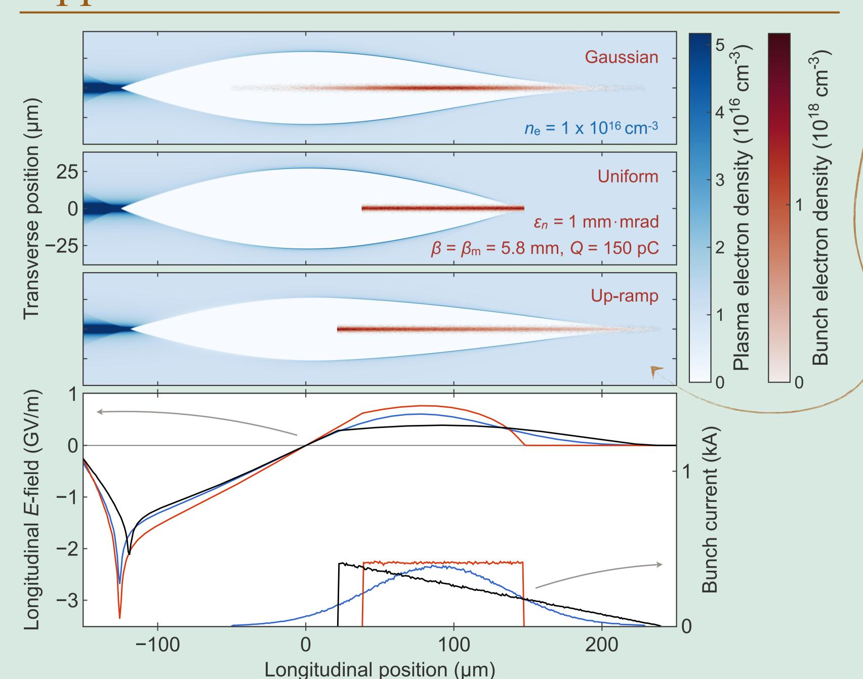
Wake-T [6] simulation snapshots. The plasmas are identical as are the bunches, apart from their current profiles (equal duration, 368 fs FWHM, like the 8.0-A setting above). The decelerating field along the upramped bunch is lowest and flattest, the accelerating fields are similar.
