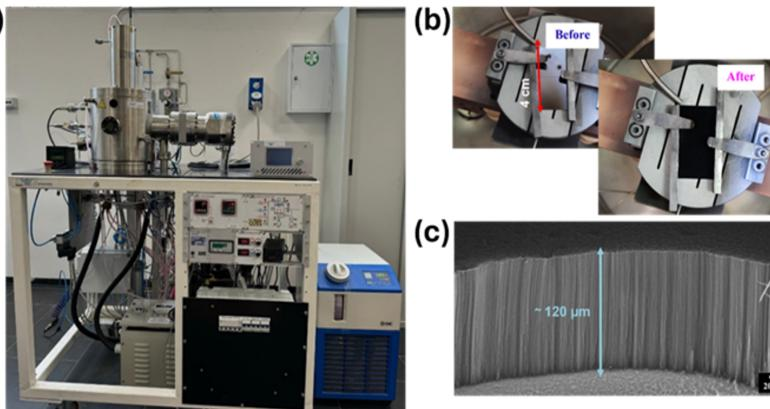
(a) The TITAN INFN-Sapienza facility at Sapienza University of Rome; (b) silicon substrate mounted on the heating element inside the CVD chamber before (left) and after (right) VA-CNTs synthesis; (c) SEM image of a typical VA-CNT array growth. G. Cavoto, et al.
