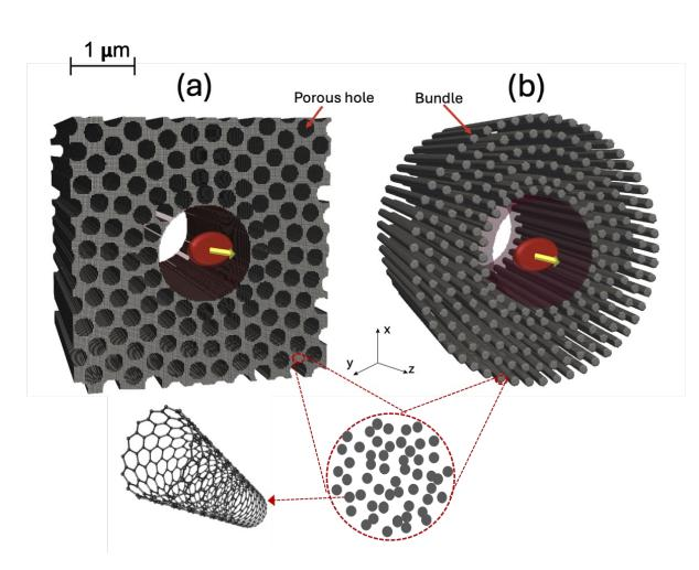
(a) porous target with walls composed of CNT bundles, and (b) nanowired target, where each wire consists of vertically aligned CNT bundles.
