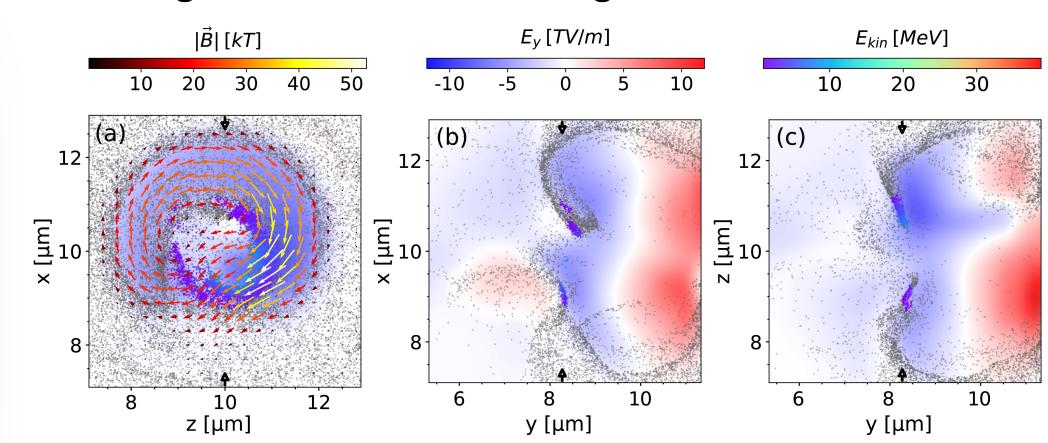
Azimuthal magnetic field peak ~ 50 kT (monitored at t/T=10)
