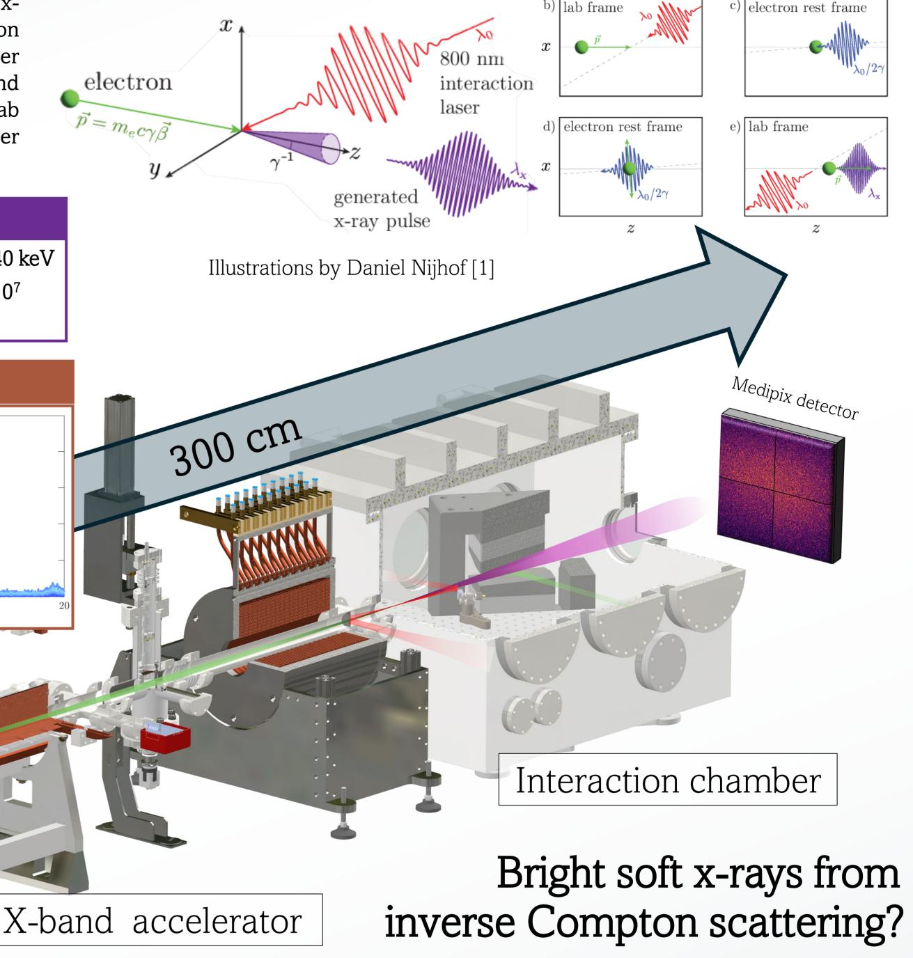
Designs for ICS sources often focus on hard x-rays. For soft x-rays ICS sources are considered to be inefficient. This inefficiency can be attributed to the low electron beam brightness owing to the low electron energy
