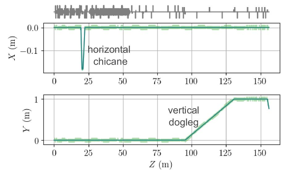
The linac features two dispersive sections for compression and collimation:
