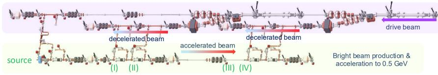
Planned multi-staged acceleration experiment to 500 MeV C. Jing et al. 10.1016/j.nima.2018.05.007 (2018)
