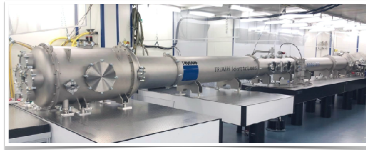
TRUMPF Multi-pass cell (MPC)* Spectral broadening
