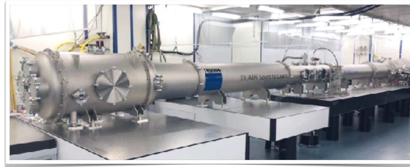
TRUMPF Multi-pass cell (MPC) Spectral broadening
