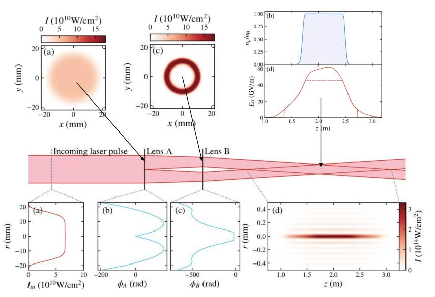
A pair of diffractive optics acts in tandem to shape the laser intensity profile.
