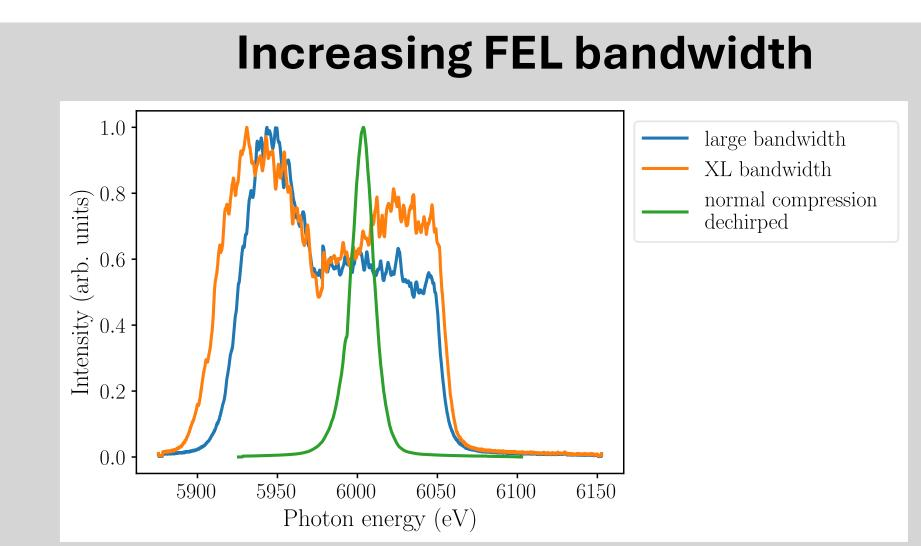
Sending overcompressed beam through the dechirpers increases the FEL bandwidth.
