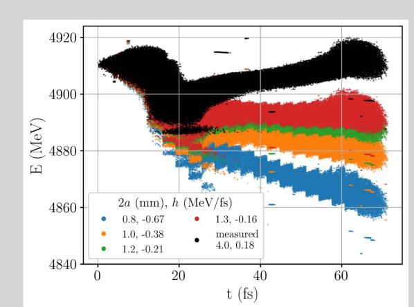
The energy spread of the beam **decreases**. For gaps smaller than ~1.2 mm, the tail loses energy such that the beam's energy spread increases.
