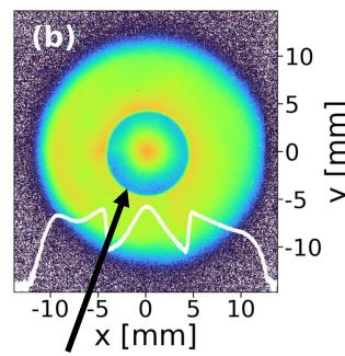
Mask allows simultaneous observation of halo and core without saturating camera
