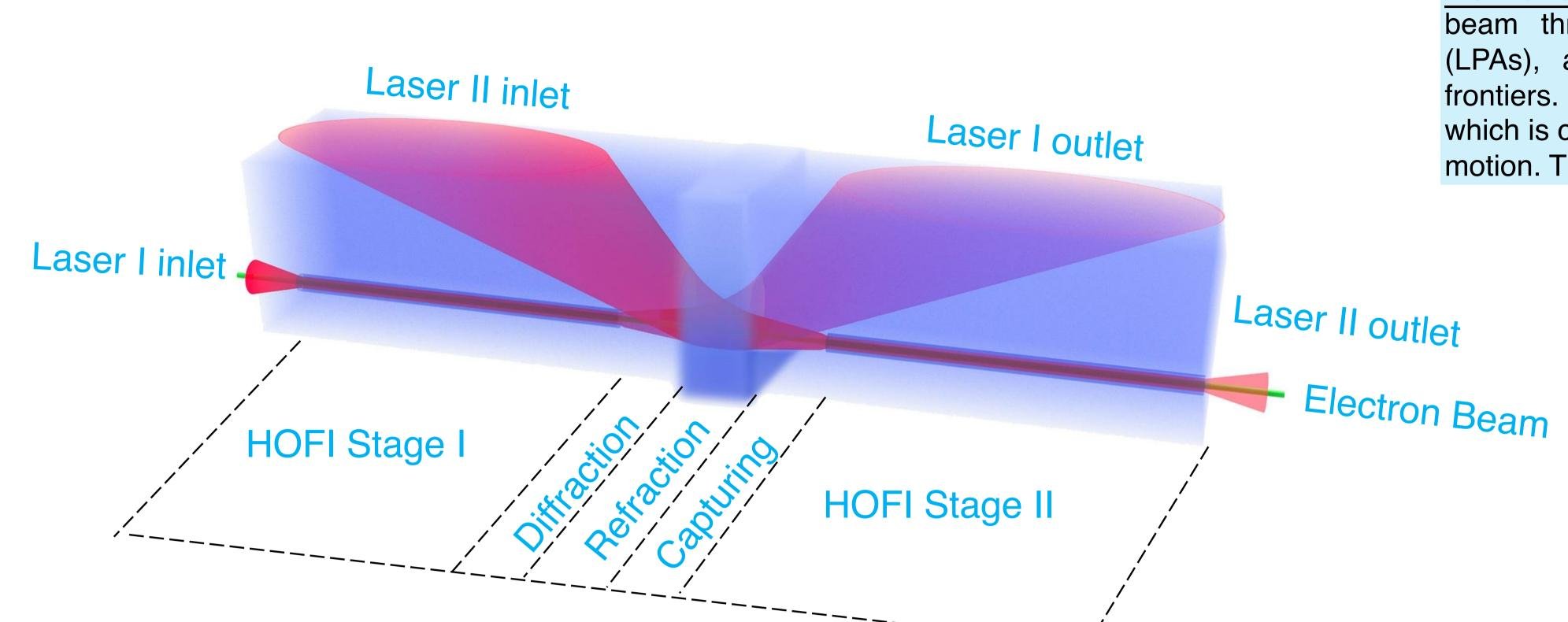
Motivation Staging consists of accelerating an electron beam through a chaing of laser plasma accelerators (LPAs), and is required to reach many-GeVs or TeV frontiers. We propose a concept of in-plasma staging, which is compact and in principle compatible with strong ion motion. This scheme is investigated with 3D simulations.
