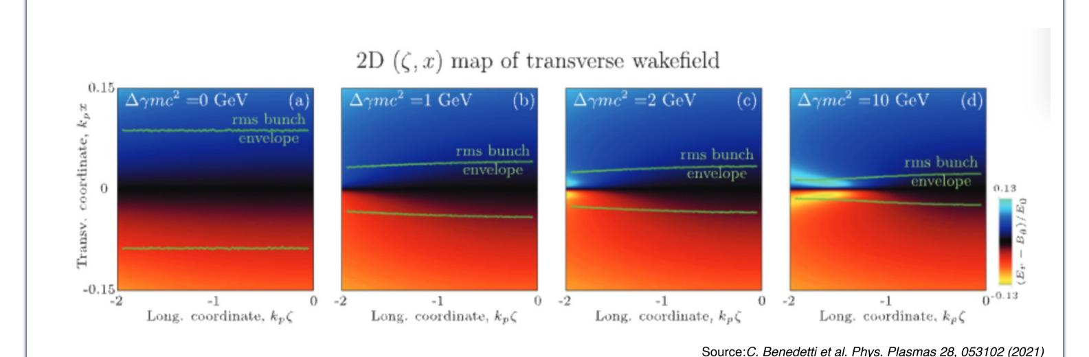
By staying in the plasma, the witness beam can be adiabatically matched to the distorted transverse field caused by ion motion.
