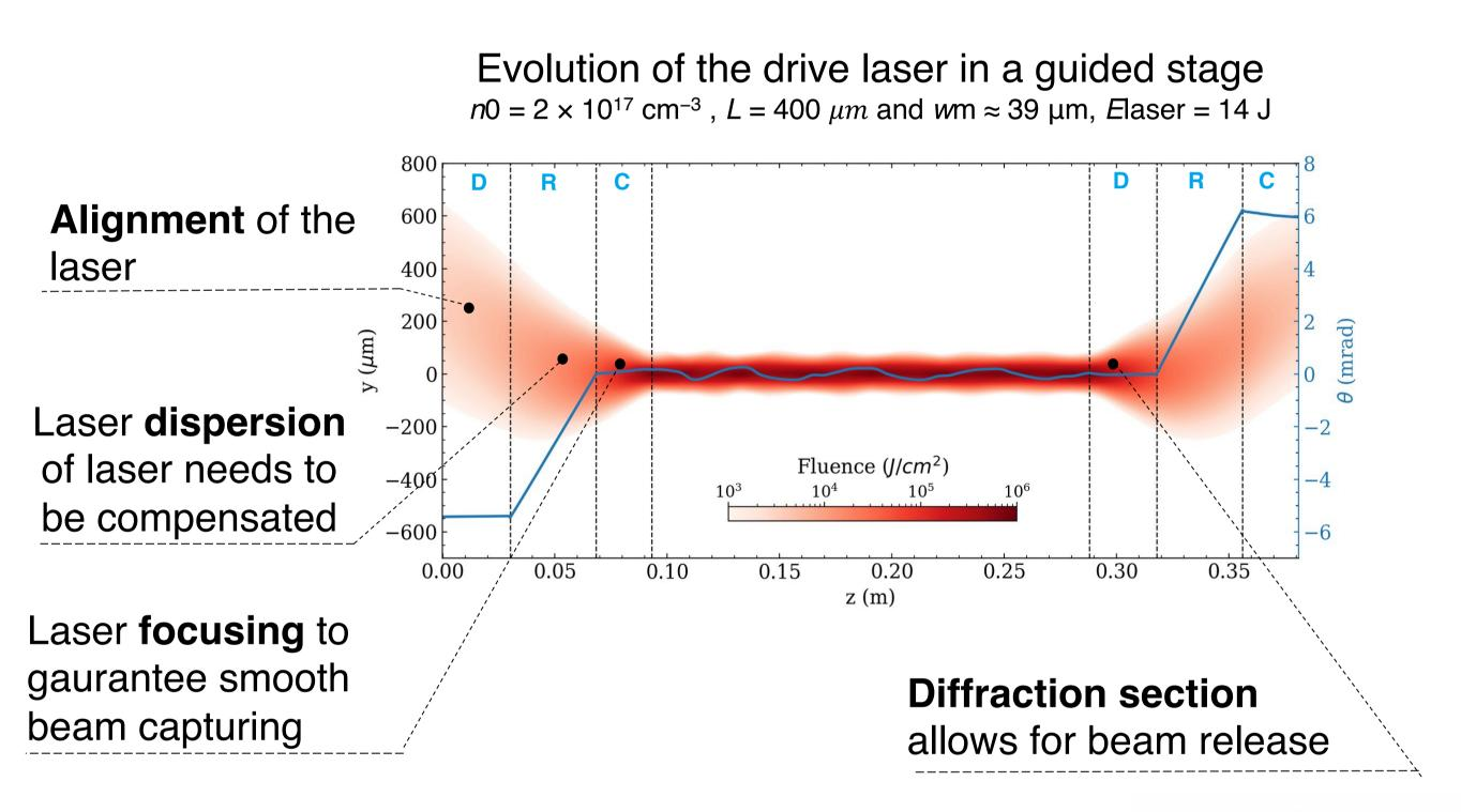
Initial laser profile is iterated through Bayesian optimization: <a href="https://example.com/linearing/linearing-nc/4">https://example.com/linearing-nc/4</a>
