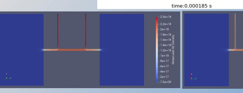
**Magneto-Hydrodynamic simulations** HD simulation results for single inlet configuration are used as a starting condition for the MHD simulation, to analyze the plasma density distribution along the capillary.
