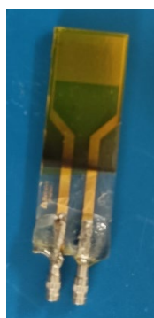
CsPbBr 3 encapsulated in PMMA
