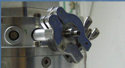
Cryostat modified to have RF ports
