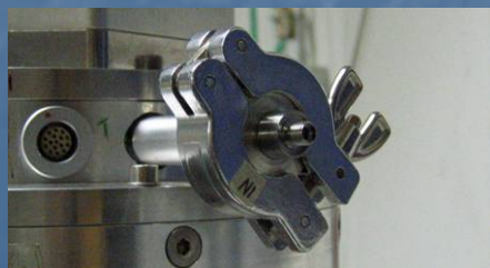
Cryostat modified to have RF ports
