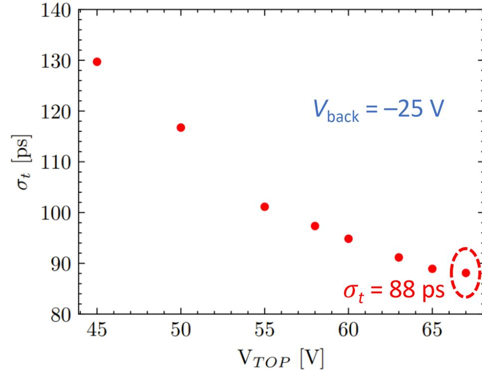
Time resolution (sensor + FE electronics) at  $V_{top} = 65$  V and  $V_{back} = -25$  V is  $\sigma_t = 88$  ps
