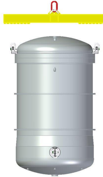
Notional lifting bar and lifting points
