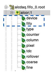
ALCOR data is decoded in a TTree structure. This is the purely ALCOR data, device and fifo are informations added later related to Beam Test configuration
