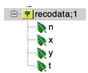
Recodata is the most filtered and analysis ready data format: each TTree event is a frame and contains the hit x, y position, the time delta (t) with the reference time\* and how many hits (n) are in the frame
