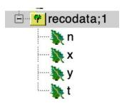
Recodata is the most filtered and analysis ready data format: each TTree event is a frame and contains the hit x, y position, the time delta (t) with the reference time\* and how many hits (n) are in the frame
