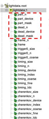
part indicates which device and FIFO is participating in the run. The device refers to the reading FPGA IP address [192-208] and the mask is a bit map for the participating FIFOs: (1001010111) > (1,4,6,8,9,10)
