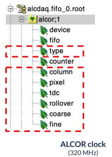
ALCOR data is decoded in a TTree structure. This is the purely ALCOR data, device and fifo are informations added later related to Beam Test configuration
