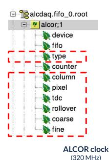
ALCOR data is decoded in a TTree structure. This is the purely ALCOR data, device and fifo are informations added later related to Beam Test configuration
