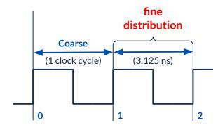
Fine distribution subdivide the coarse counter (clock cycle) into roughly ~70 parts bringing down the resolution potentially to ~45 ps
