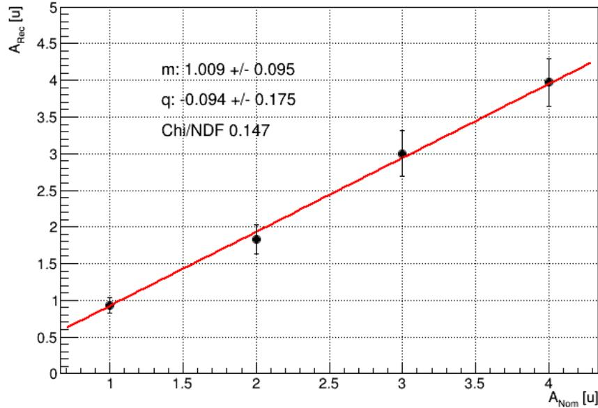
For Z up to 4,  $A_{\text{rec}} / A_{\text{nom}}$  ratio is  $\approx 1$ .
