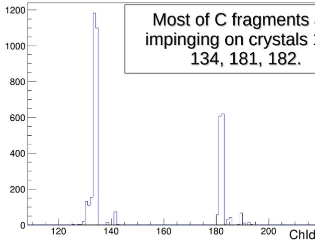
Most of C fragments are impinging on crystals 133, 134, 181, 182.
