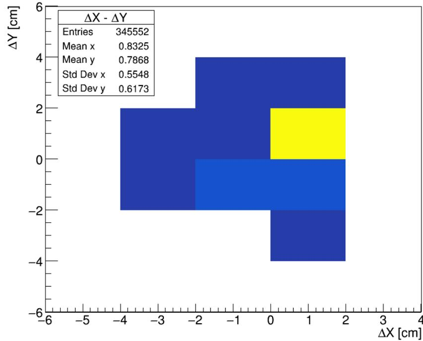
After calibrating the clusters, their position is shifted, in most cases between up to 2 cm in both axis → within CALO granularity.
