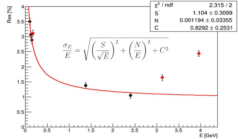
Data acquired during CNAO2024 were fitted with this usual 3-parameters function, in order to obtain a resolution vs E function
