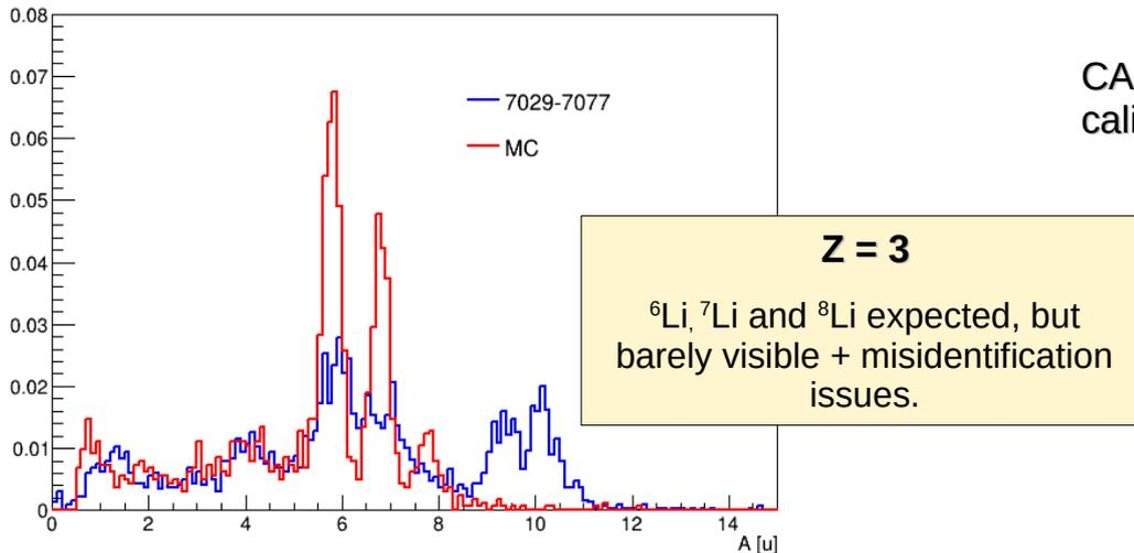
CALO resolution was modeled according to CNAO24 calibration points and added to MC simulation.
