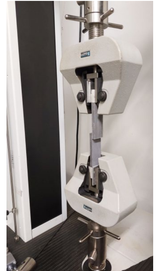
Single lap shear test ISO 4587-2003
