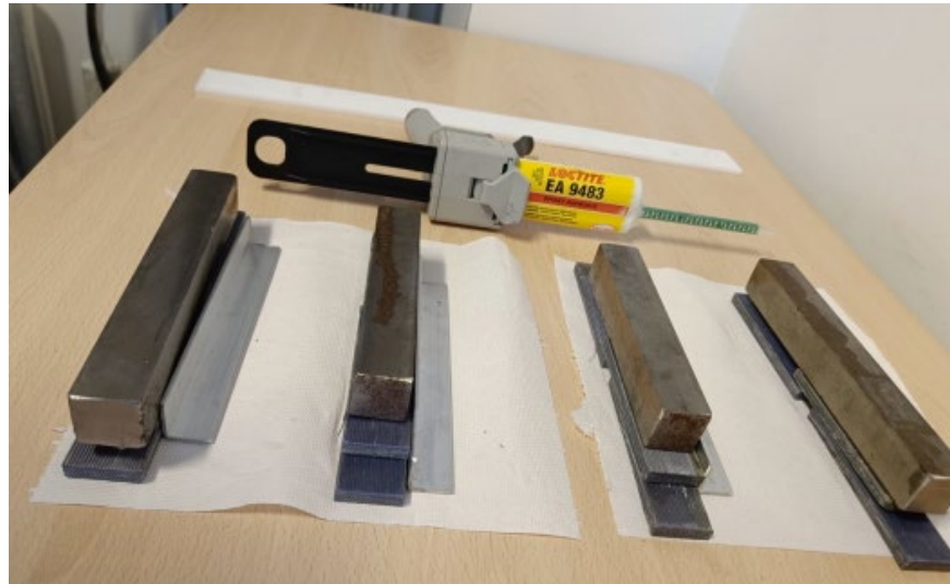
specimen for glue tests
