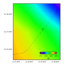
Geoidal undulation (The black spots are the traverse stations along the tunnel)
