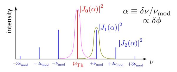
Excite <sup>229</sup>Th crystal with detuned VUV laser  $\nu_{\rm laser} = \nu_{\rm Th} + \nu_{\rm mod}$  and compare to on-resonance excitation  $\nu_{\rm laser} = \nu_{\rm Th}$
