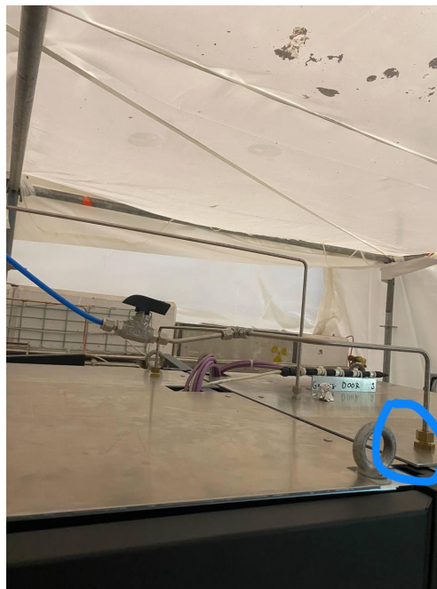
Air leak at mixer
