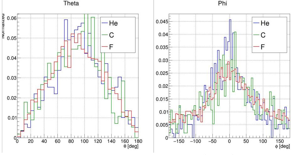
Theta and phi are the recoil directions in the laboratory reference frame
