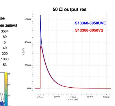
Avalanche begins  $\rightarrow$  switch is closed,  $C_d$  discharges through  $R_d$  with time constant
