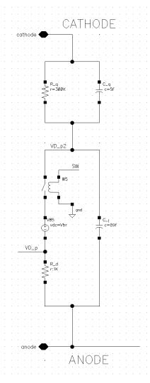
Avalanche begins  $\rightarrow$  switch is closed,  $C_d$  discharges through  $R_d$  with time constant
