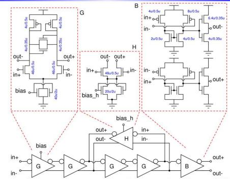
Very fast comparators are obtained by cascading low-gain cells. Full CMOS levels generated only in the last stage.
