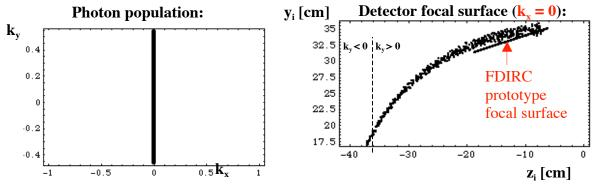
In the region, where the FDIRC prototype works ( $z \sim -6$  cm), the calculated focal plane is close to a straight line. So our solution with a flat window was OK. Our results would be perfect for  $k_x = 0$  of the detector plane would have zig-zag shape.
