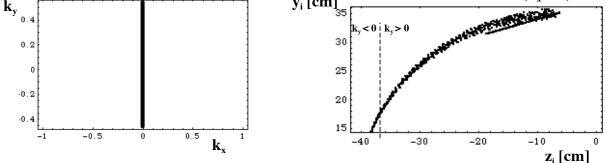
In the region, where the FDIRC prototype works ( $z \sim -6$  cm), the calculated focal plane is close to a straight line. So our solution with a flat window was OK.
