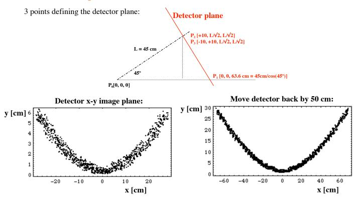
**Indeed, there is a periodic kaleidoscopic pattern even without a mirror.** It is created by the square bar. To see it better, move the detector plane back by 50 cm. Since the wiggles originate from the bar, i.e., the mirror has nothing to do with it, it cannot be easily fixed.
