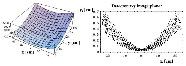
**Note:** Based on the Vellum program of the FDIRC prototype, expect for  $x_f \sim -20$  to 20,  $y_f \sim 35$ ,  $z_f \sim -(3-6)$  in the bar coordinate system. The calculation is not that far from the expected numbers.
