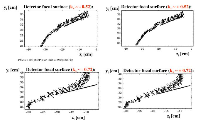
The detector surface shape is changing as a function of  $k_x$ , mainly as  $k_y$  is approaching 0, which corresponds to photons going parallel to z axis.
