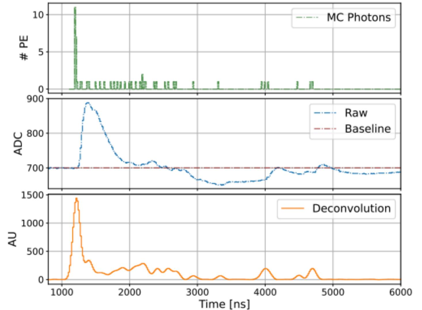
Waveform deconvolution to remove the signal bipolarity introduced by our AC-coupled readout
