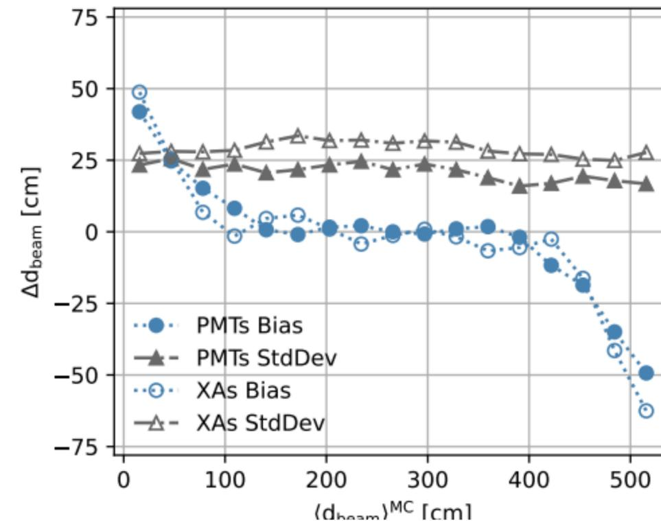
Bias and resolution in the estimation of the interaction point in the beam direction (Z) for the PMTs (full marks) and X-ARAPUCAs (empty marks) flashes
