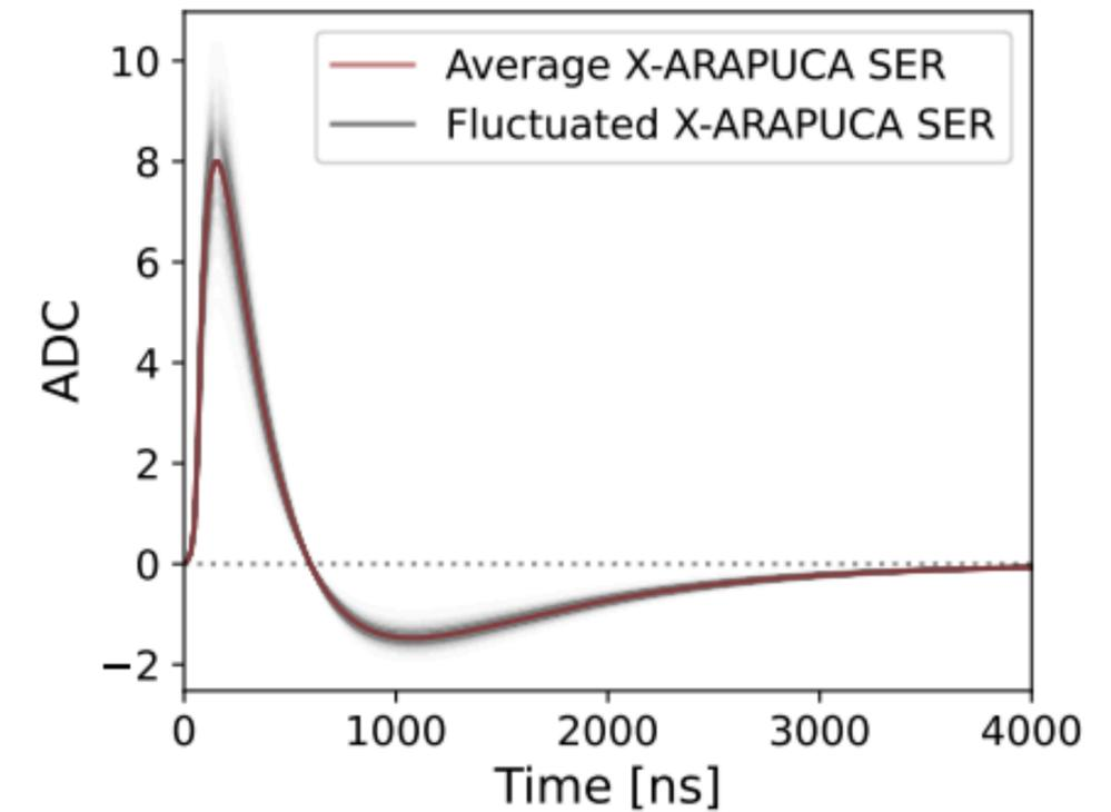
Measured Single Electron Response for the PMTs (Left) and X-ARAPUCAs (Right) in SBND
