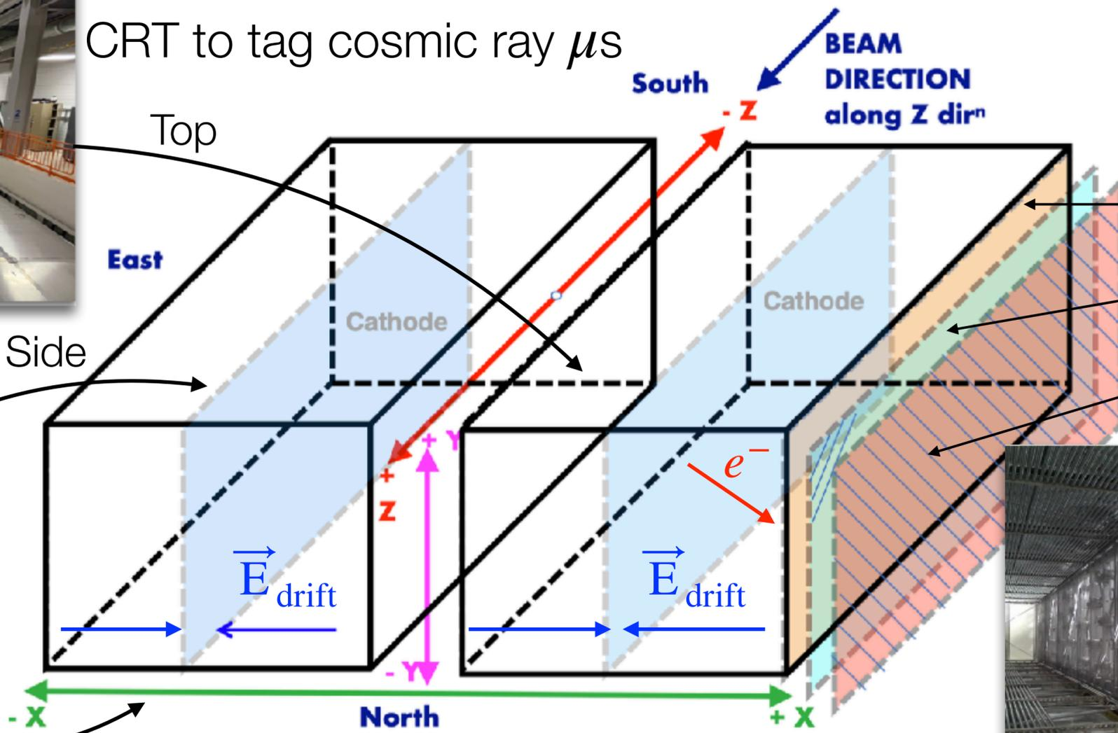
Ionization charge read by 3 wire planes with different orientation:
