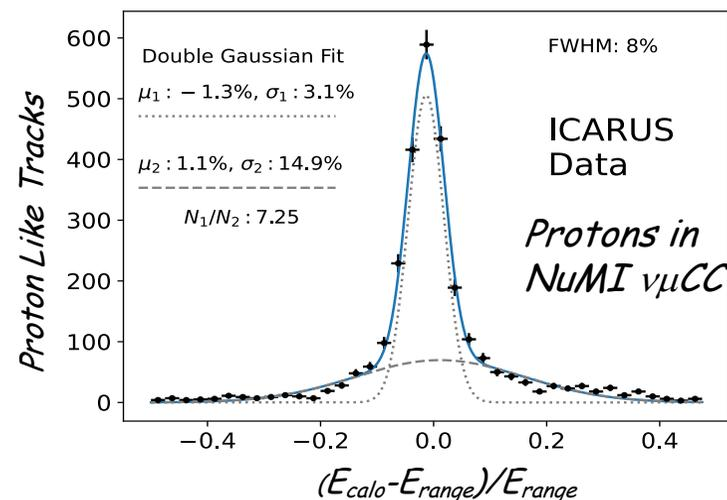
*Difference between calorimetric and range measurement of the proton energy*
