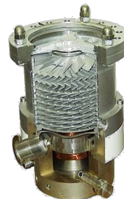
Interior view of a turbomolecular pump
