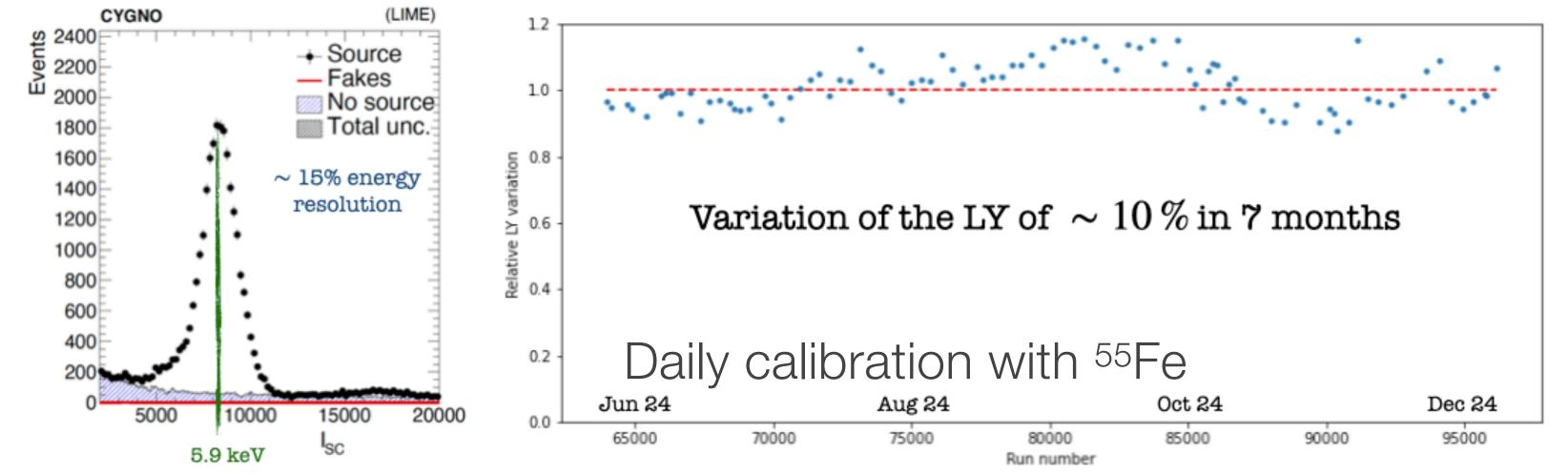
Detector calibration with <sup>55</sup>Fe is now a completely automated procedure and showed a stability with 7% RMS over 6 months
