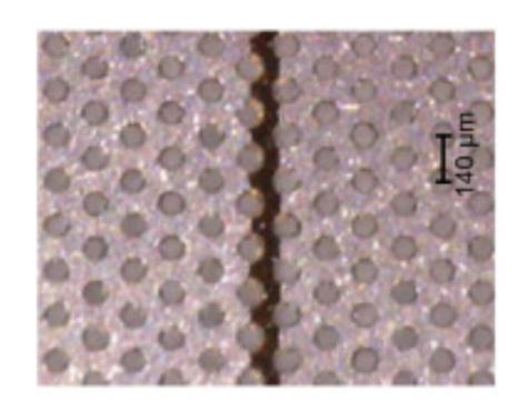
Random **segmentation** should reduce the dead area while keeping the operational stability (tested by CMS-GEM)
