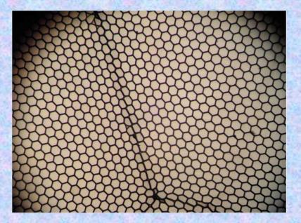
Incom substrate, 40µm pores, 8 deg bias, 40:1 L/D, 83% OAR
