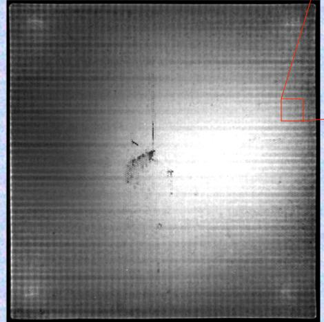
**20cm MCP pair image with 185nm UV illumination The central defect is unique to one MCP batch.** III Seminario Nazionale Rivelatori Innovativi 21
