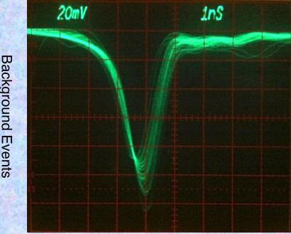
ALD borosilicate MCP pair, 20µm pore, 60:1 L/d, 8° bias, 0.7mm/1000v MCP gap. Single event pulses are ~1ns wide. ~Typical response for 20µm pore MCPs.
