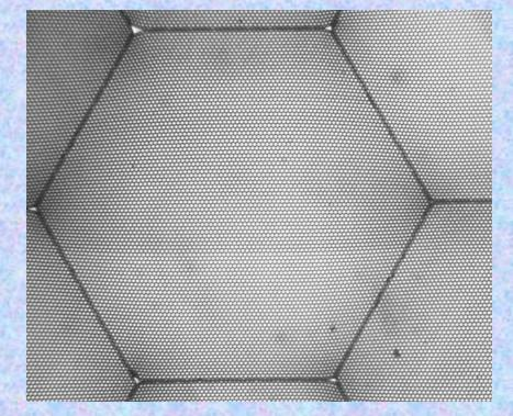
Photo of a 20µm 65% OAR, 8° bias, 60:1 L/D, finished substrate, prior to ALD coating.
