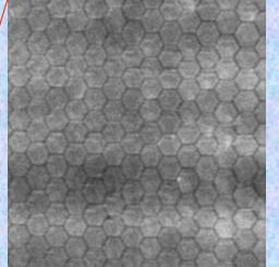
Image section showing the MCP multifibers Spatial resolution ~100µm FWHM.
