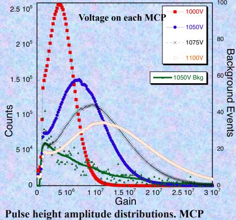
Pulse height amplitude distributions. MCP pair, 20µm pores, 8° bias, 60:1 L/d, 0.7mm pair gap with 300V bias. 3000 sec background.
