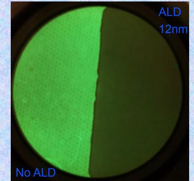
1100v MCP, 2700v Screen, UV flood Photonis ML201-B-2 MCP, 90M $\Omega$
