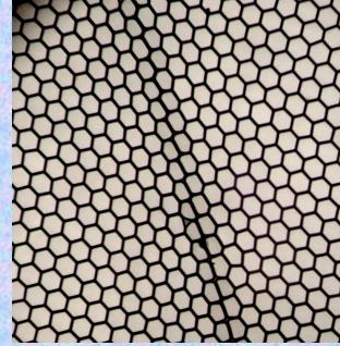
40µm pore borosilicate microcapillary MCP with 83% open area.
