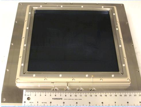
20cm ALD 20µm pore MCP pair in detector assembly with a cross delay line imaging readout.
