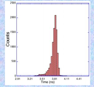
Laser (~80 ps) measurements of timing jitter show 100ps time spread, 25mm cross delay line readout, 10µm MCP Z stack, S20 photocathode
