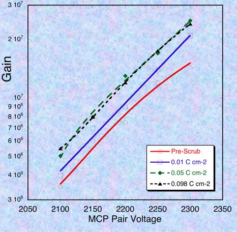
UV scrub gain curves for ALD MCP pair 180-141 (20µm pore, 60:1 L/d, 8° bias).
