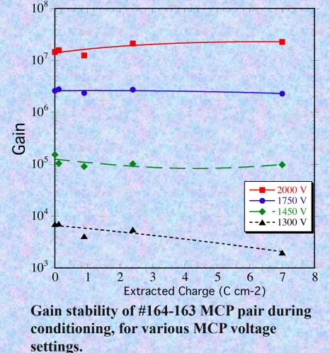
Absolute gain curves for MCP pair with NO vacuum bake. Gain rises with use!
