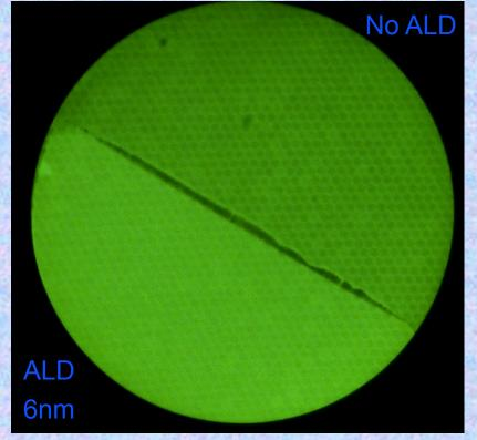
1150v MCP, 2800v Screen, UV flood Photonis ML201-B-1 MCP, 86MΩ
