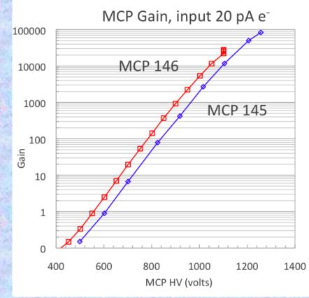
Single MCP tests in DC amplification mode show imaging and gain very similar to conventional MCPs. Sample imaging performance has improved dramatically with substrate and ALD coating process improvements.
