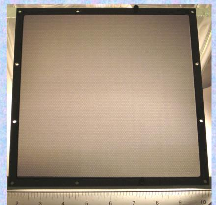
20cm MCP showing the multifiber stacking arrangement, 40μm pore, 8° bias.
