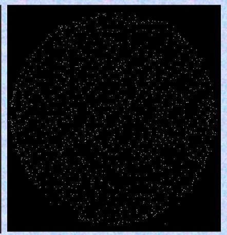
3000 sec background, 0.0845 events cm<sup>-2</sup> sec<sup>-1</sup> at 7 x 10<sup>6</sup> gain, 1050v bias on each MCP. Get same behavior for most of the current 20μm MCPs.
