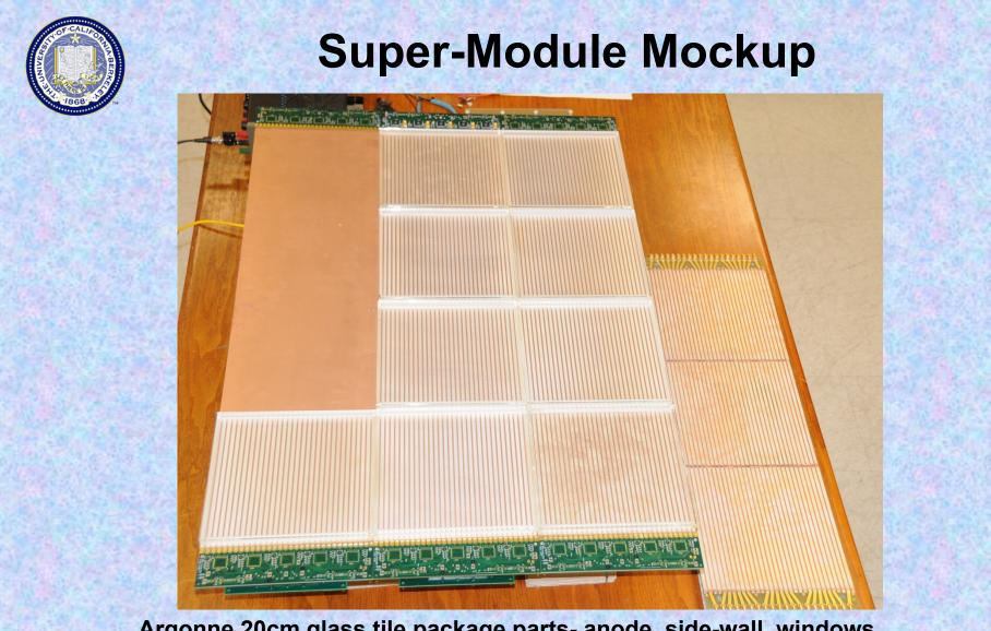
Argonne 20cm glass tile package parts- anode, side-wall, windows Shows the stripline anodes (no MCPs)
