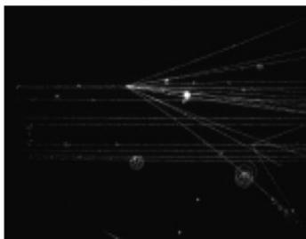
The dry ice keeps the bottom very cold – so that the vapor, once it has fallen, is in a so called supercooled state. This means, the alcohol is in vapor form, but at a temperature at which vapor normally can't exist. It is, as if you had made steam at 95°C. Since the vapor is at a temperature where it normally can't exist, it will very easily condense into liquid form if anything disturbs its equilibrium.
