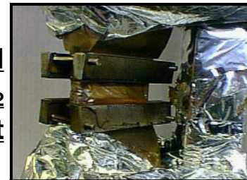
Typical liquid H 2 target
