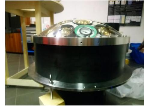
Implosion test relevant to investigate if any implosion of 50cm PMT can affect the mPMT vessel (cracks or damages) and its fixing in the frame. We did not expect an implosion of the mPMT
