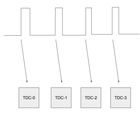
each test pulse is recorded by a different, subsequent TDC reconstruction of pulse period requires calibration of all TDCs global minimisation calibration approach
