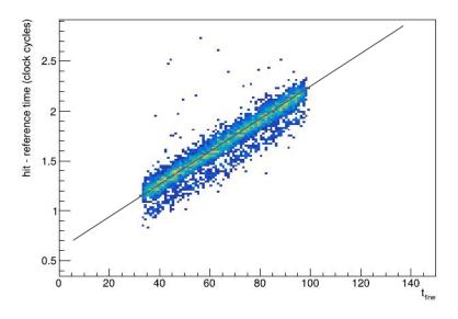
if the test pulses are sent asynchronous to the ALCOR clock, we can uniformly populate the full  $t_{fine}$  range uniformly, unless non linearities in  $t_{fine}$  binning of ALCOR TDCs
