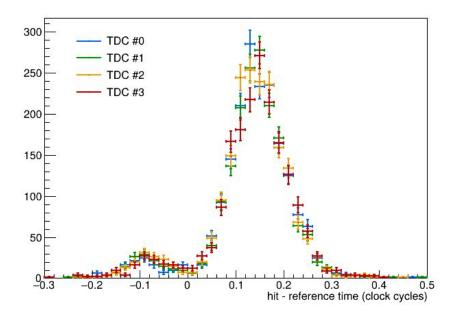
this plot was obtained with nothing else more than the TDC calibration obtained with test-pulse data and a common offset to bring it closer to zero
